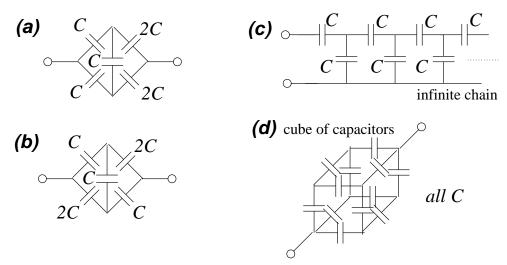
Use symmetries of the configurations to calculate their total capacitances.
